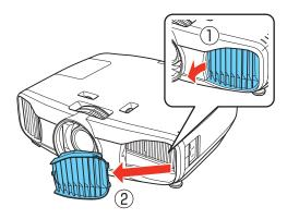
4. Remove the air filter as shown.
